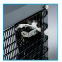
FloodGuard - inlet solenoid only opens to allow water into the cooler, when water is dispensed. By remaining closed all other times it protects the cooler against leaks. (On POU coolers only)
